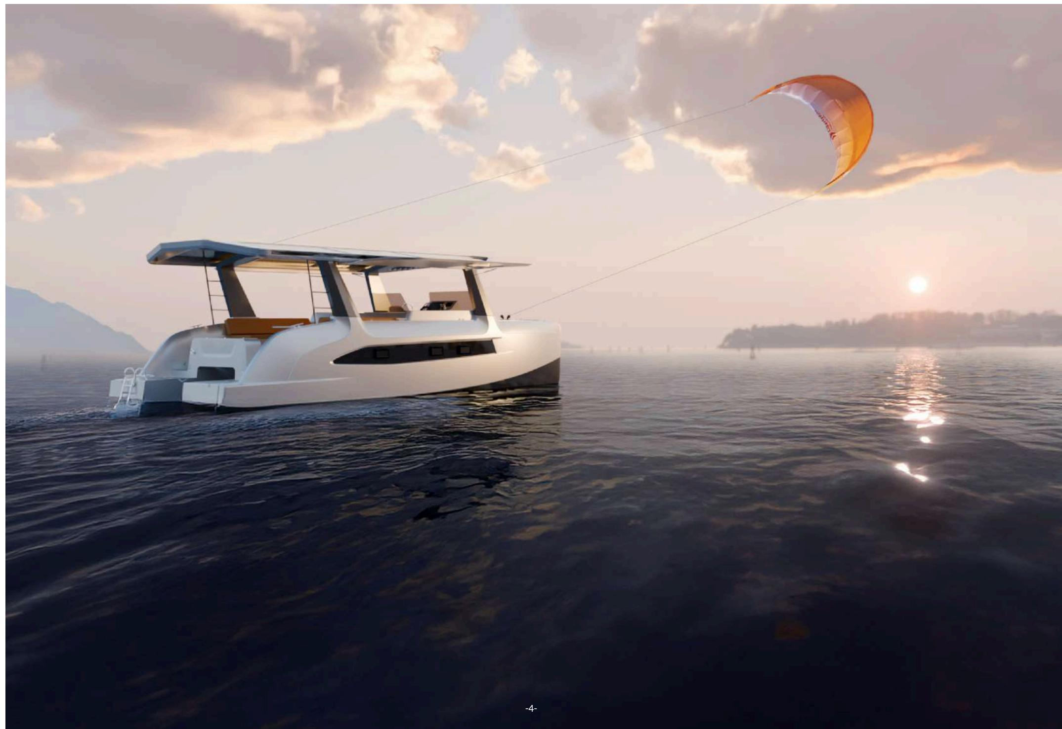
The M.10 has been designed with autonomy and comfort in mind. Equipped with solar panels on its roof and foldable side wings, it offers near-unlimited autonomy in full sunlight. The bifacial panels utilize water reflection to capture up to 20% additional energy.
